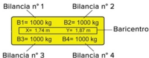
Suitable for creating wheel weighing and static axle weighing systems, or to weigh objects with various resting points. Ideal for weighing and calculating the centre of gravity coordinates of the vehicles, trucks, airplanes, containers, etc. Simultaneous display of the weight of each connected pad and of the sum. CE-M approved (OIML R-76 / EN 45501).
