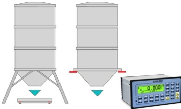
Software for 3590EXT and CPWE weight indicators, to create single product dosage systems in loading (useful for filling hoppers, silos or big bags, or guiding the operator in the manual dosages) and in unloading (useful for dividing the quantity of materials of equal weight or extract precise quantities from the silo, with management of the reloading). Database of 500 formulas.
