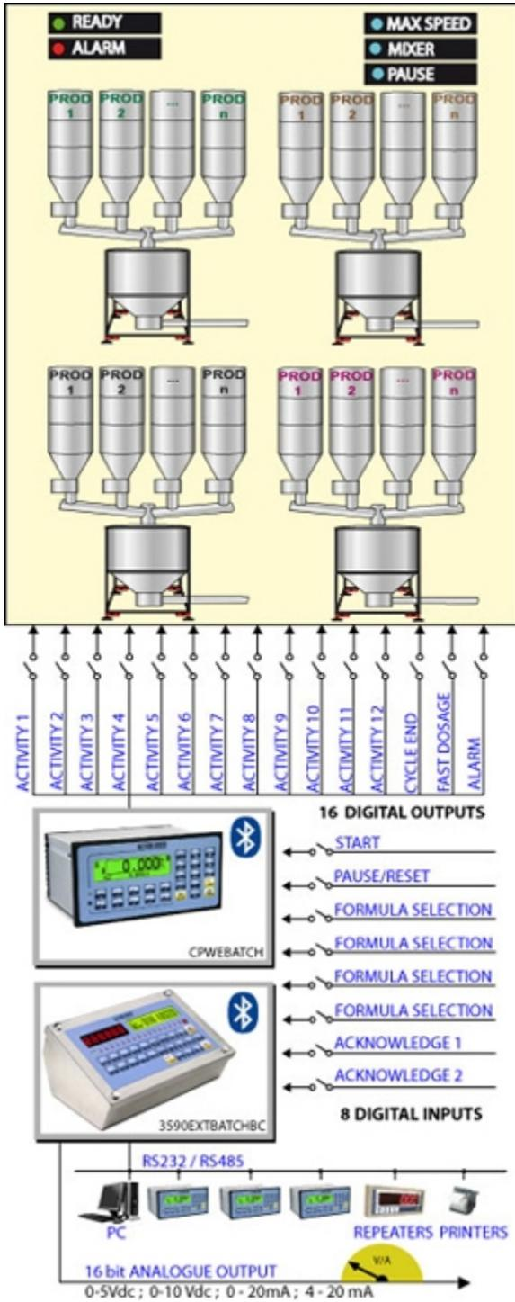
Software for multicomponent dosage with various scales, for CPWE and 3590EXT indicators.
