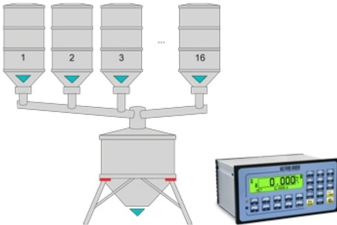
3590EXT and CPWE weight indicators software version for automatic multicomponent and multi scale dosage systems. Database of 100 different activities and 500 formulas. Direct management of 12 different components through the relay. Completely programmable printouts.
