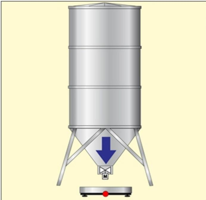
Configuration which allows to manage a dosage system in loading of a single product, useful for filling hoppers, silos or big bags, or guiding the operator in the manual dosages.
