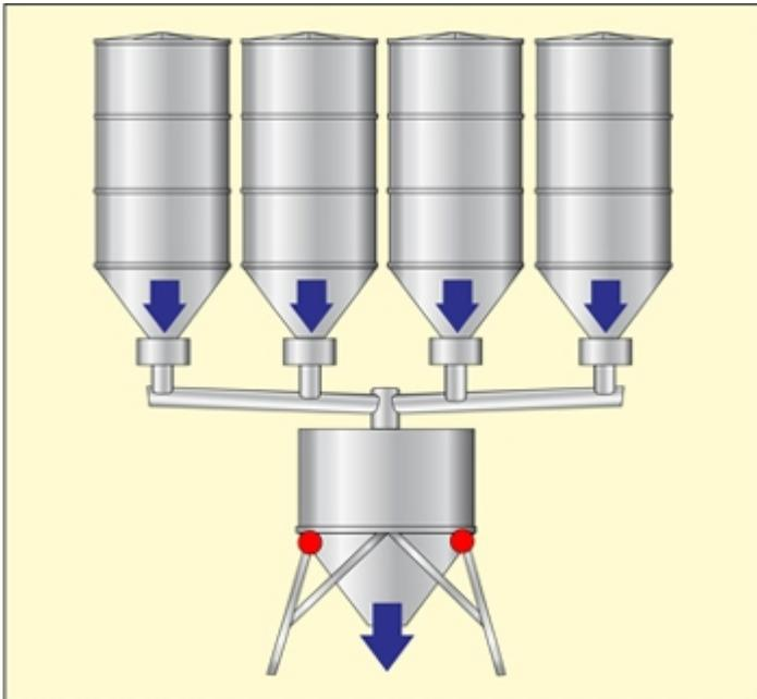
Configuration which allows the dosage of various products, in loading or unloading, as well as mixing and formulation, with the possibility of managing mixers, burners or vibrators using dedicated contacts.
