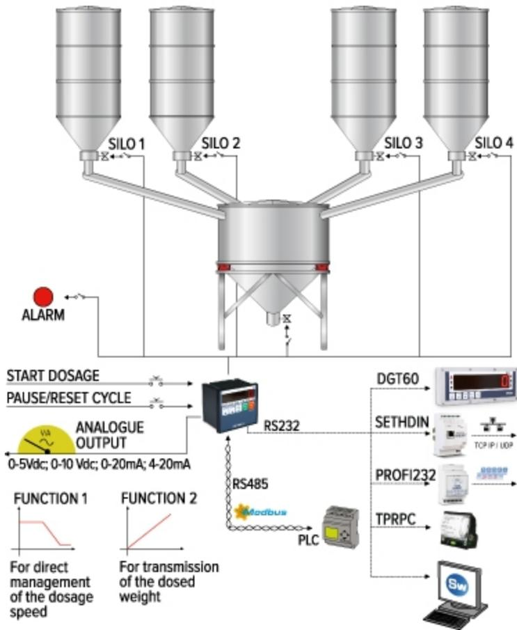
Example of dosage system using the DGTQF for loading routine
