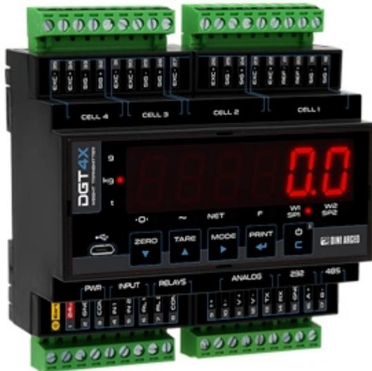
Weight transmitter for weight transfer to PLC via fieldbus, analog output or RS485. It allows the reading and diagnostics of each load cell or each connected scale.
