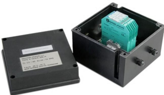
Kit of three intrinsic protection Zener barriers, for connection of devices in ATEX area with devices in safe area, housed in an ABS box.
